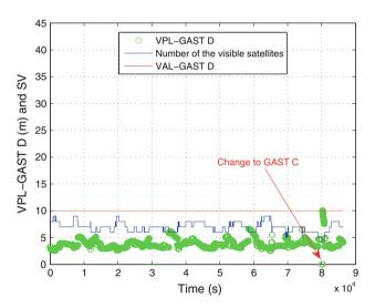
Fig. 7 Simulation results of single point for GAST D (GAST D at Point 3-Case 2)
