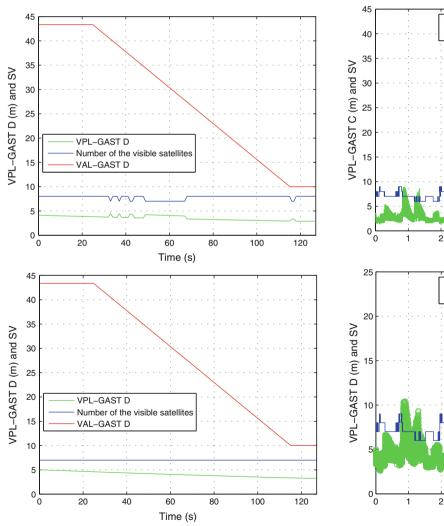
**Fig. 8** Impact of the filter initialization time of 200 s on newly rising satellites. Filter initialization time not considered (*top*), filter initialization time considered (*bottom*)
