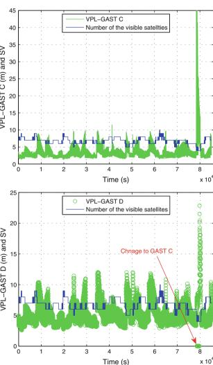
**Fig. 9** The VPL and number of the visible satellites (initialization time 200 s is considered). GAST C Case1 (*top*), GAST D Case 1 (*bottom*)
