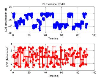
Figure 15: Received signal amplitude and phase with the DLR channel model, with 90° of azimuth angle
