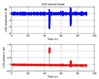
Figure 13: Received signal amplitude and phase with the DLR channel model, with  $0^{\circ}$  of azimuth angle
