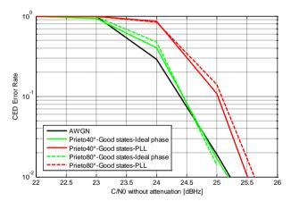
Figure 19: Demodulation performance of GPS L1C with the Prieto channel model forced to generate only good states
