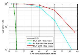
Figure 17: Demodulation performance of GPS L1C with the DLR channel model with  $0^{\circ}$ ,  $45^{\circ}$  and  $90^{\circ}$  of azimuth angles
