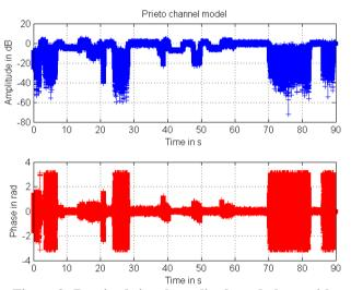
Figure 9: Received signal amplitude and phase with the Prieto channel model
