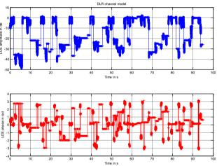
Figure 14: Received signal amplitude and phase with the DLR channel model, with 45° of azimuth angle
