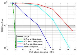
Figure 18: Demodulation performance of GPS L1C with the Prieto and the DLR channel models with an ideal phase estimation
