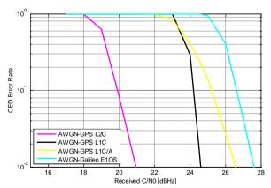
Figure 8: Demodulation performance of GNSS signals in the AWGN channel model with the classical methodology
