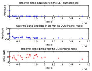
Figure 12: CIR example of the DLR channel model, with 90° of azimuth angle
