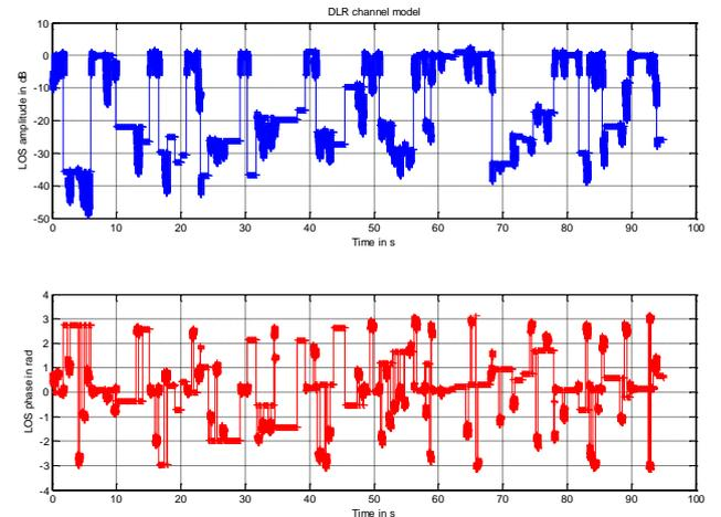
**Figure 14: Received signal amplitude and phase with the DLR channel model, with  $45^\circ$  of azimuth angle**
