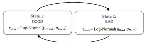
**Figure 3: Semi-Markov chain state transitions process**
