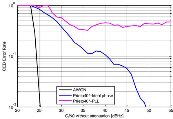
**Figure 16: Demodulation performance of GPS L1C with the Prieto channel model**
