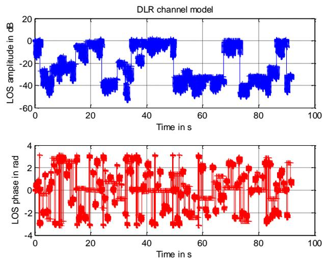
**Figure 15: Received signal amplitude and phase with the DLR channel model, with 90° of azimuth angle**
