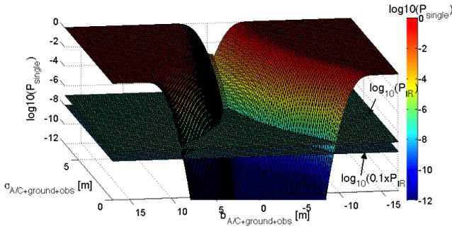
**Figure 10: probability of positioning failure given a Gaussian ranging error  $N(b_{A/C+ground+obs}, \sigma_{A/C+ground+obs})$  on a single pseudo range measurement – control during parking on the apron**
