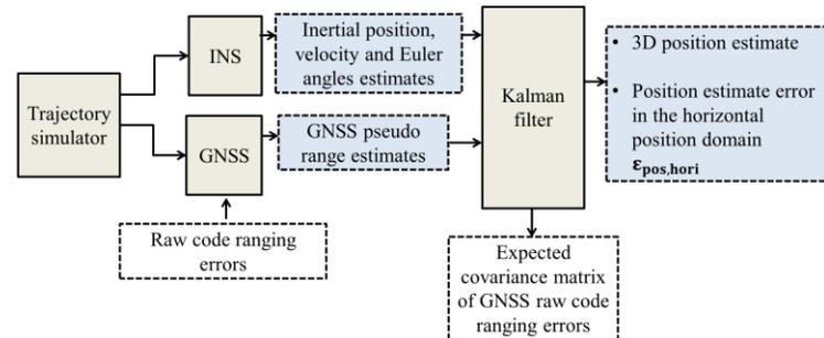
Figure 1: Architecture of the position estimate error simulator
