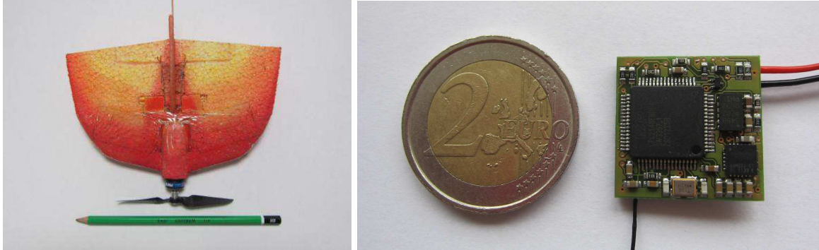
Figure 5: The prototype QUARK MAV with the new developed QUARK Paparazzi Autopilot (October 2012)
