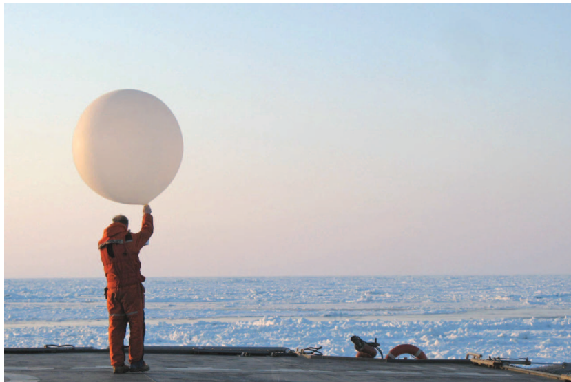
Figure 8. Launch of a radiosonde (RaSo) from the coast guard vessel KV Svalbard.
