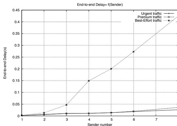
Fig. 3. Average End-to-end Delay vs. number of Senders
