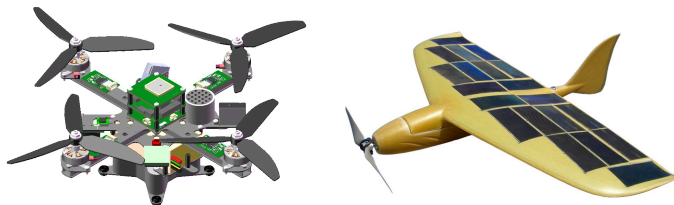
Figure 1. Quadrirotor (Blender, 350mm diameter and 300g weight) and aircraft (Solar Storm, 500mm span and 400g weight) min-UAVs from the ENAC (Ecole Nationale de l'Aviation Civile) University
