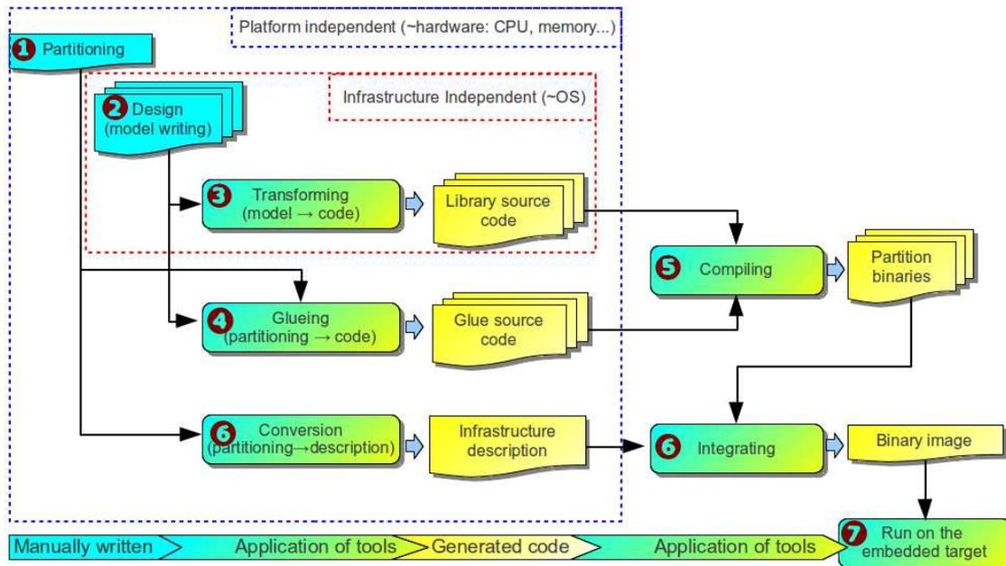
Figure 1. Development methodology for software fast prototyping
