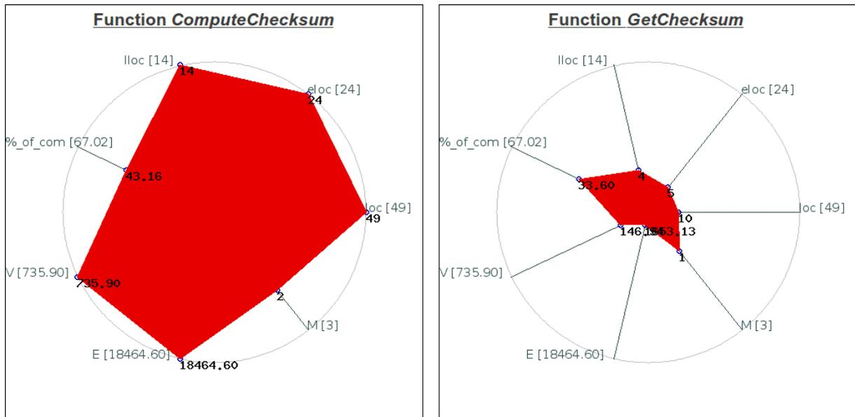
**Figure 3. Signatures of the functions ComputeChecksum and GetChecksum**
