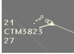
Figure 9 : the comet of an evolving aircraft, the image exhibits direction and acceleration changes
