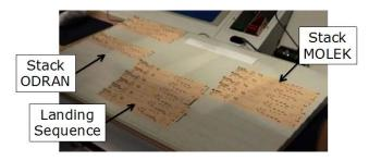
**Fig. 2.** The flight strips on the strip board are organized into three groups. The upper left and right groups contain the strips for aircraft in each of the two stacks. The centre group holds the strips for the aircraft that have left the stack and are approaching the runway beacon.
