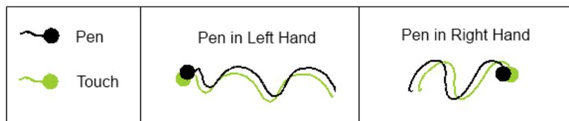
**Fig. 6.** When the pen in held is the right hand the light from the pen is detected to the right of the pen tip. When the pen is held in the left hand the light is detected to the left of the pen tip.
