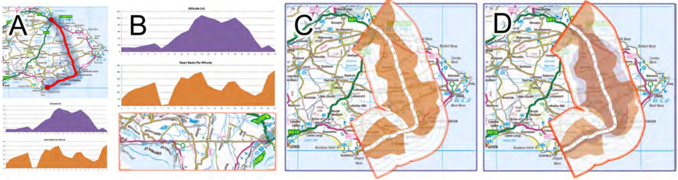
Figure 1. A) Cycling data: a map with a route and area graphs with average altitude (purple) and heart-rate (orange) at each kilometer. B) The rectified route map aligned under the linear graphs enables comparison of the measured variables to the map features. C) The heart-rate graph wrapped around the route in the map shows effort in spatial context. D) Same as C, but with multiple variables. Map used contains Ordnance Survey data © Crown copyright and database right 2013.
