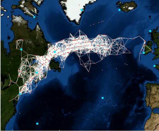
Figure 2. AANET Connectivity in Oceanic Area
